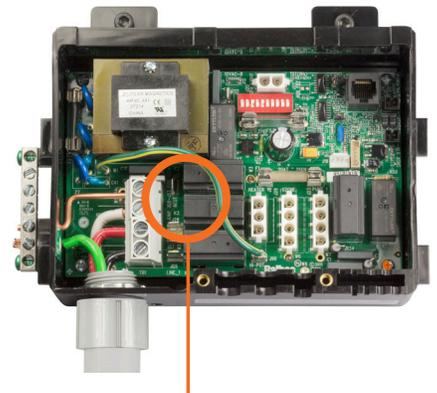
The wire jumper is removed from a 240V system.
