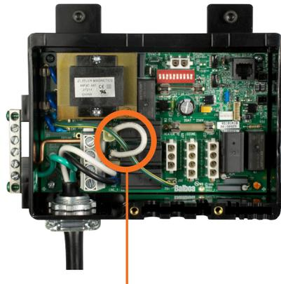
The wire jumper connects J28 and J57 on a 120V system.
